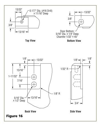
Route notch in top corner of overlay panel as shown (see Top and Side Views). Top of notch is entire depth of panel, front to back.
